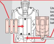
Use a Phillips/cross head screwdriver (not included) to loosen screw in battery compartment door (screw remains attached to door). Remove door and discard old batteries. Insert 3 x 1.5V fresh "AAA" or R03 size batteries. Alkaline batteries recommended. Replace door and tighten screw.
